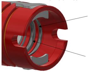
3. Lubricate new main seals with Krytox and install into grooves. No tools required to perform installation.
